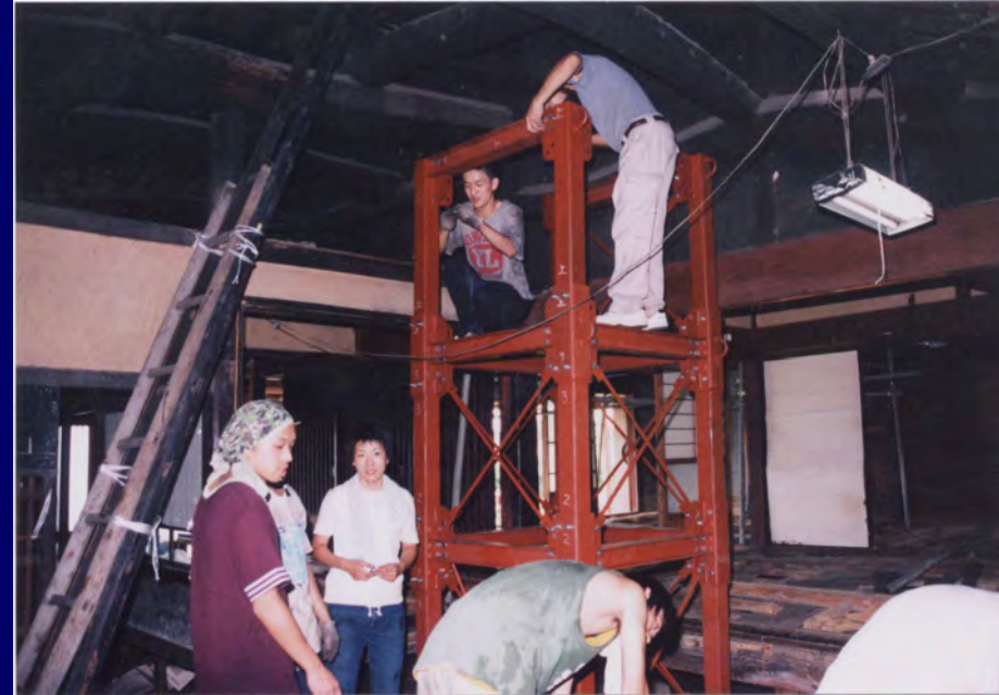
Static loading test on existing house, 2000
